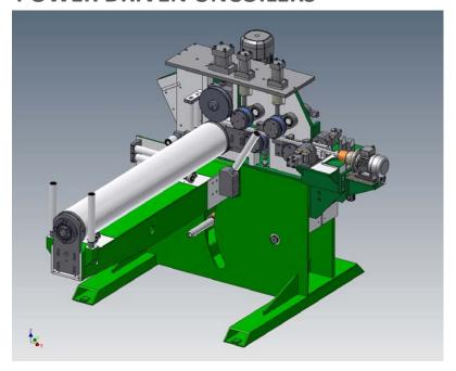
They are used for UNCOILING and STRAIGHTENING the wire for cold formers, nut formers and bolt makers.
